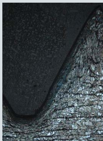
転造ねじ Cold-formed thread
